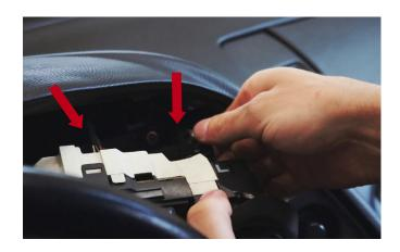
Disconnect the wires from the RH warning light pods and the emergency blinker button.
