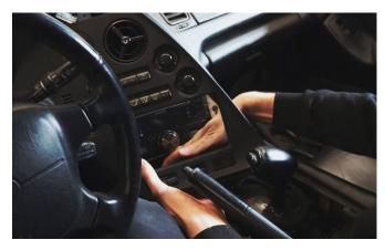
Unplug all the connectors from the backside of the panel.
