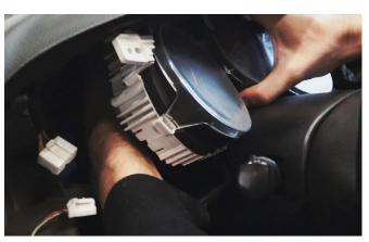
Take out the cluster a bit, carefully and unplug all connectors on the back. (There's 2 or 3 connectors)
