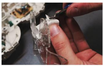
Cut it off with flushcutters, and remove the excess.
