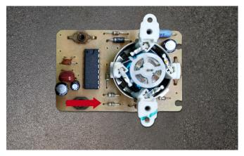
(For JDM 180km/h clusters, repeat the process for the Speed motor PCB, with the shown resistor.
