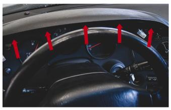
Next up, remove the 5 screws from the top dash panel and pull it out.
