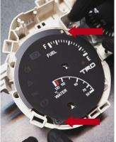
Repeat for the TACH and fuel gauge fase. Use the guides for aligning and press down the face.
