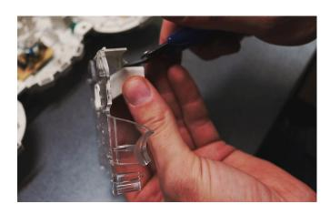
Remove the top plastic part. It's in the way for the new LED panel.
