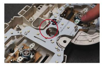
Make sure the cable goes upwards and doesnt interfere with anything on the back.
