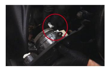
Plug in the dimmer and mount the panel. (This is only temporarily for testing, therefore no need to plug in every connector at this moment)
