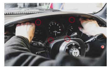
Grab the cluster shroud dash panel and pull it out. It is mounted with 4 clips.
