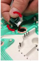
If it still doesnt light up, take out the cluster and turn the light fitting 180° and plug it back in so that the polarity is reversed.
