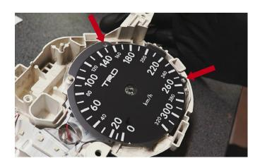
Now, align the pins on the acrylic cover, with the holes on the faces and stick the face down. Press where the tape is.
