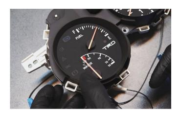
When satisfied with the position, fully seat the temperature needle.
