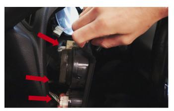
Unplug the connectors and remove the panel.
