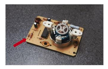
Replace the shown resistor, with the one included in the kit. It's in the bag with the remote.
