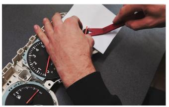
This way you can pride the needles up, without scratching the faces. Use the plastic clip remover for priding up the needles.
