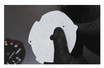
Take you new speedometer face and one of the needles you just removed and insert it into you new face.
