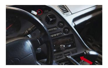
Remove the radio panel. It's held in place by one screw and clips.
