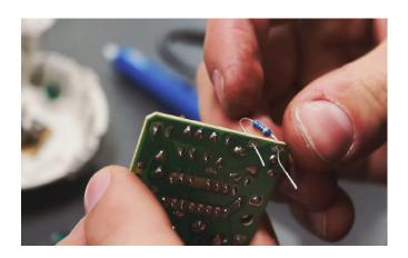
Make sure both holes are clear, and insert the new resistor.
