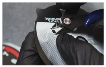
The needles are just melted into place from the backside. Squeeze in carefully the melted plastic so you can pull the needle out.
