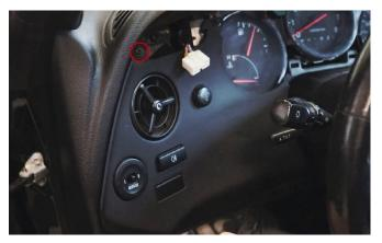
Next, remove shown dash panel. Remove the top screw and pull the panel out. It's held in place with clips.
