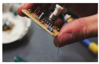
Pull the resistor all the way down. Its not polarized, (no + and - ) meaning you can put it in, in any direction.
